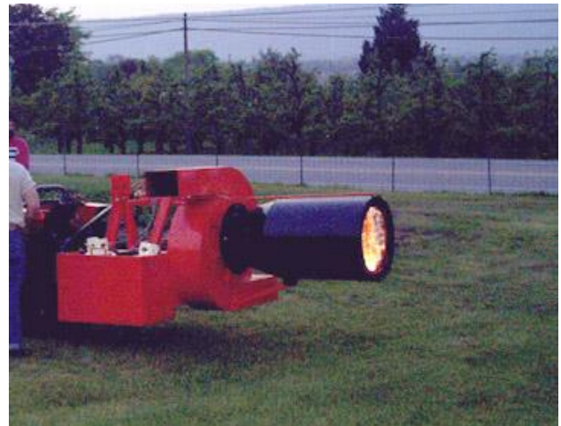
Figure 4.7 Frost Protection Using a Mobile Propane Heater (Photo by R. Crassweller).
